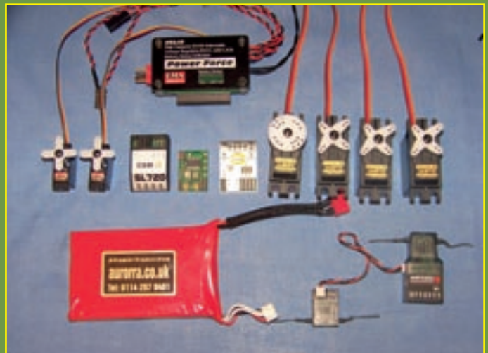
Radio gear comprises a mixture of JR and Hitec servos, CSM 720 gyro and Aurora Revolution 4500 3c 2s LiPo battery pack
