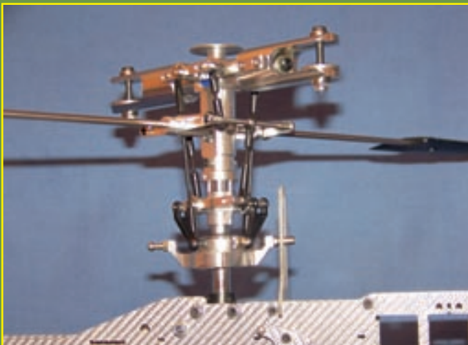
The completed rotorhead installed on the X-Treme main frame
