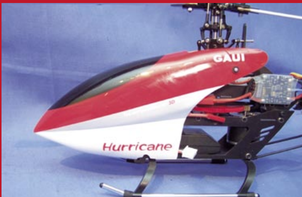
The electronic speed controller was added to the upper frame which allowed for a neat cable run
