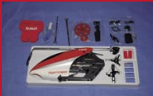
The Gaui 200 V2 semi kit requires some assembly
