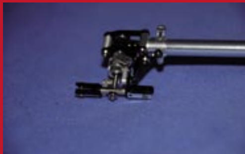
The tail of the V2 features a new pitch control system
