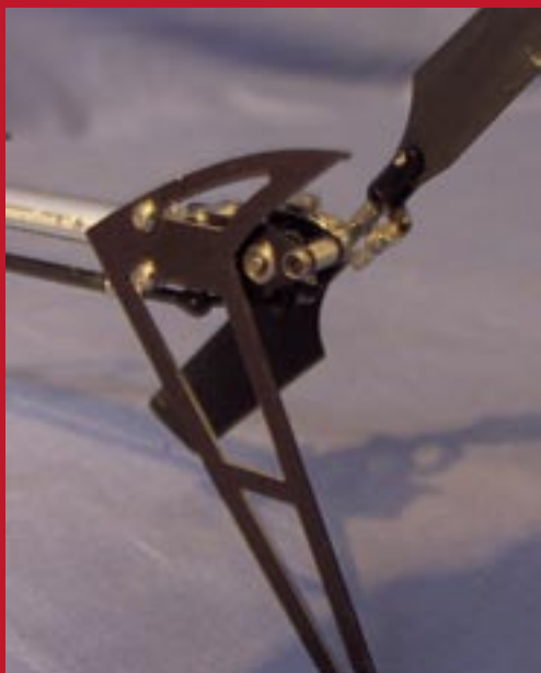
The heli has an alloy tail boom and G10 tail fins
