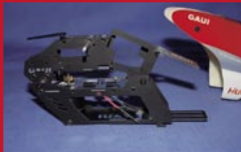
The main frames of the V2 are now made from G10
