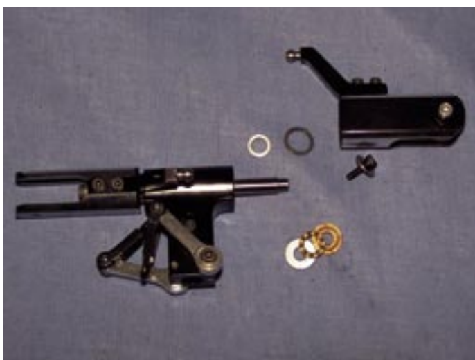
The CNC alloy head block, blade grips, pitch arms, driver arms and thrust races
