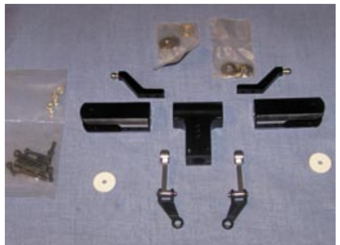
The RJX kit contains plenty of CNC machined and black anodised alloy parts
