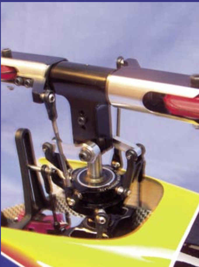
A close-up of the RJX flybarless conversion parts fitted to our test 500
